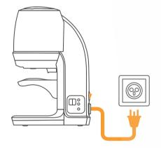
1. Insert power cable and turn on PUQpress. The tamper base will move to the upper position.
