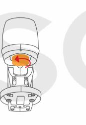
**5.** Remove tamper base by turning counter-clockwise.
