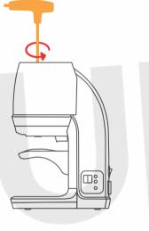
**3.** Unscrew by turning counter-clockwise.
